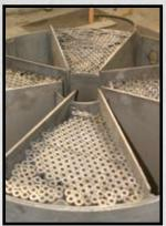
The final step to producing a precision Bergara Barrel is the stress relieving process. This high temperature heating process realigns the steel molecules ensuring that the barrel is free from any stress after the button rifling process.
