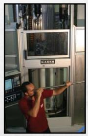
Most other barrel manufacturers move from deep hole drilling to reaming, a process that leaves tool marks in the bore. Instead of reaming, Bergara uses three separate honing spindles that utilize diamond tipped bits. These bits polish the barrel's interior surface to a mirror-like finish without tool marks.
